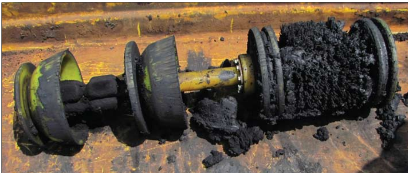
An 8-in. Enduro Cleaning Pig Train equipped with cups, scraper discs, wrap brushes and magnets retrieves solid debris from a natural gas line that was rarely pigged. Magnets and brushes are saturated with debris, resulting in additional cleaning runs.
